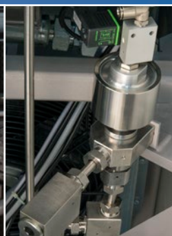
External control of the bleed down valve for piercing process.
